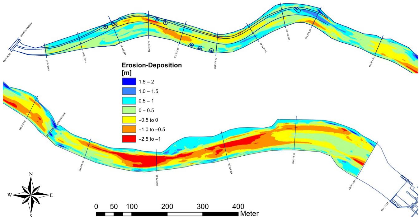
**FIGURE 2** Bed level changes (difference map Oct 2005–May 2006) for the upper part of the reservoir Bodendorf, red indicates erosion, blue deposition
