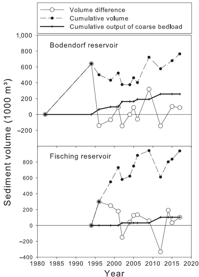
**FIGURE 4** Trend in total sediment volume (zero = start of operation), volume difference between echo sounding surveys, and output of coarse bed load for Bodendorf and Fischeing reservoirs
